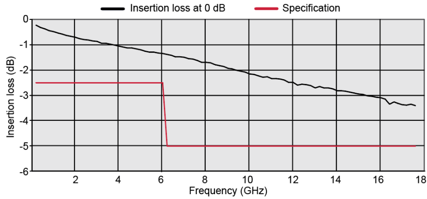
Figure 6. Keysight J7211B attenuation control unit insertion loss (at 0 dB) versus frequency
